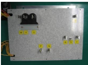
9. 티센동양 CV-60 POWER STACK
