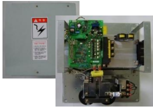
1) 티센동양 DY-20 POWER-STACK 100A
