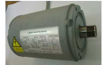
8) LG-OTIS, 도어모터, 3상,80W,4극, 29Hz,80V,1.5A
